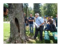
Ed Hayes finishing a demo sample with an F-400 Resistograph of the south side of the maple's lower stem. Removal in time was the recommendation for this maple. Both easy and advanced decay detection tools are used during the field training. Attendees have the opportunity in the field to make assessment decisions and try out the tools, this photo by Levy Tree, Duluth, MN.
